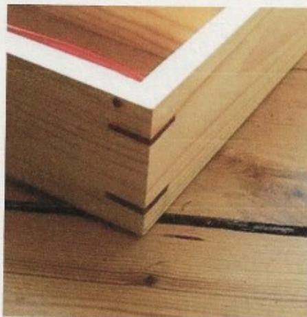
Photo 6 - Spline placed 90 degrees to the Miter
