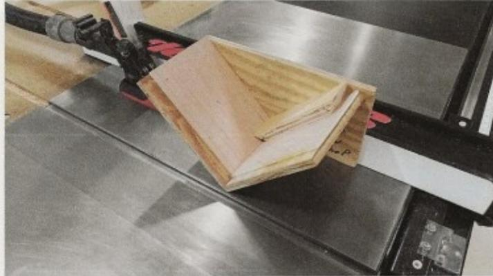
Photo 7 - Box Making Spline Jig #3
